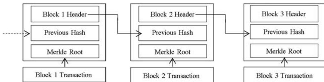
FIGURE 10.6 The structure of a blockchain.
