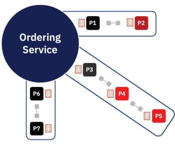
The **Ordering Service** is responsible for receiving transactions from **peers**, organizing them into blocks, and distributing the blocks back to the appropriate **channels**. Once the **peers** within a **channel** receive a block from the ordering service, they will add it to the blockchain that they jointly manage.
